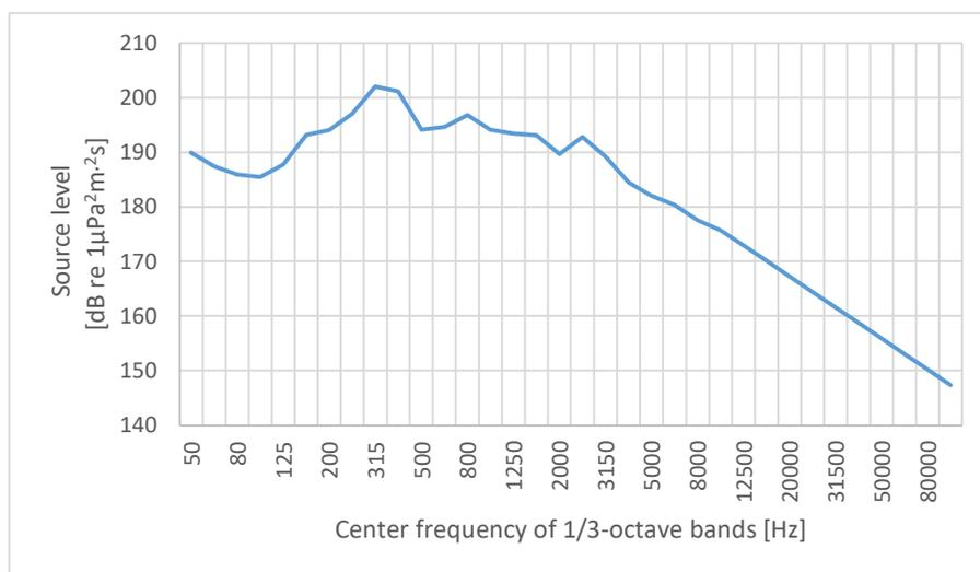
**Figure 20. Source level 1/3-octave spectrum for pile driving, stated as  $L_{S,E}$ .**
