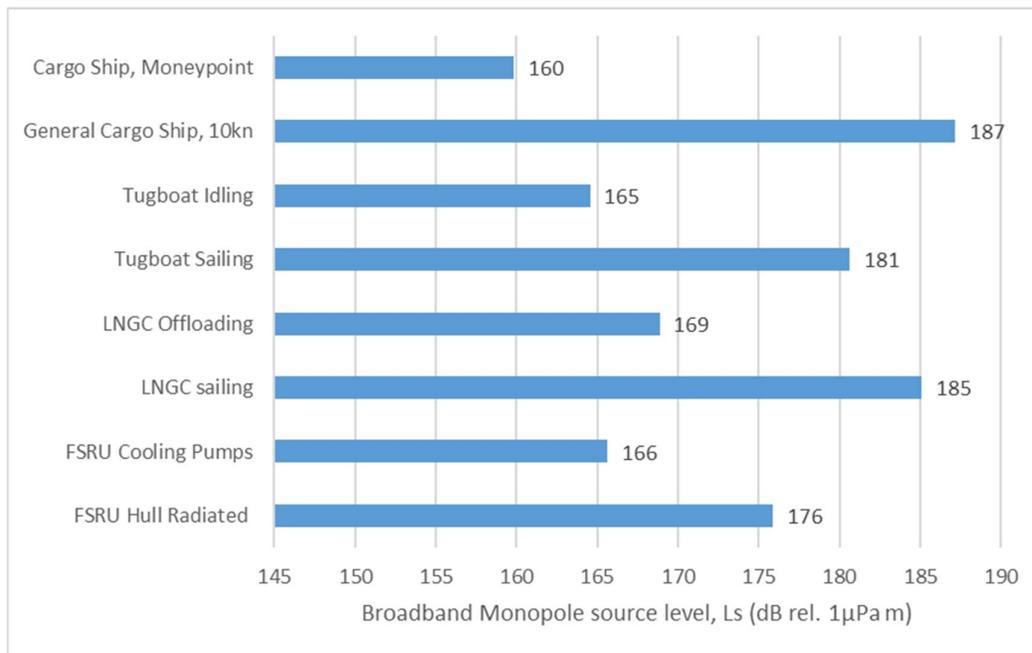
**Figure 31. Broadband underwater source levels for ships used in the predictions ( $L_s$  dB re  $1\mu\text{Pa}\cdot\text{m}$ )**
