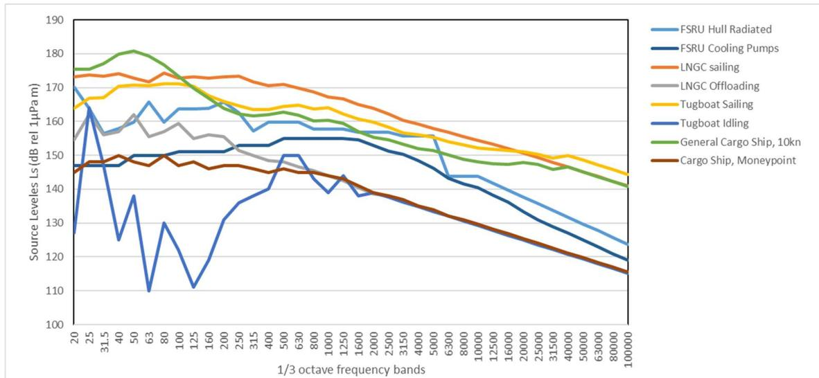
**Figure 30. Underwater source levels for ships used in the predictions ( $L_s$  dB re. 1  $\mu\text{Pa}\cdot\text{m}$ ).**
