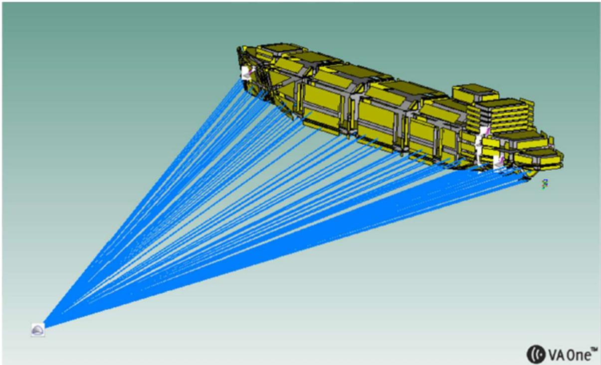
Figure 44. Picture of VAOne model of the Golar Igloo (exploded view).
