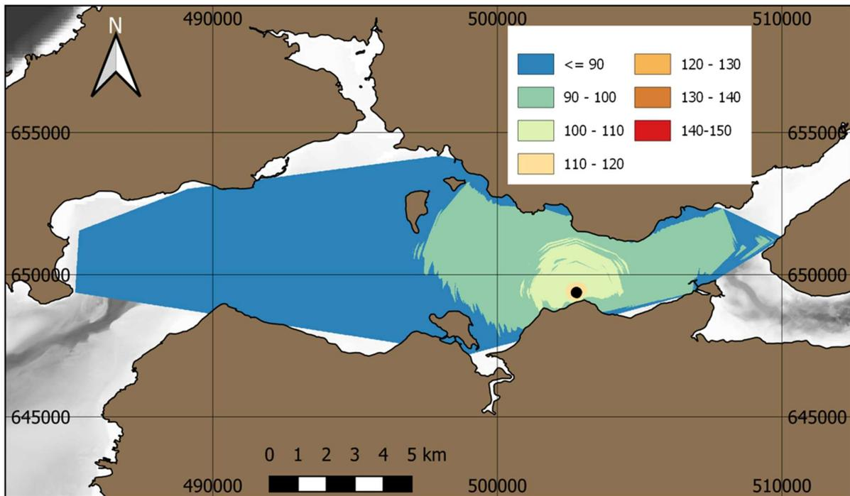
**Figure 32. Scenario A) FSRU with onboard seawater pumps. Contour map of  $L_{p,rms}$  (MF-weighted, “Max-over-depth”). Values in dB re  $1\mu\text{Pa}$ . Behavioural criteria of 120 dB is indicated by dashed line.**
