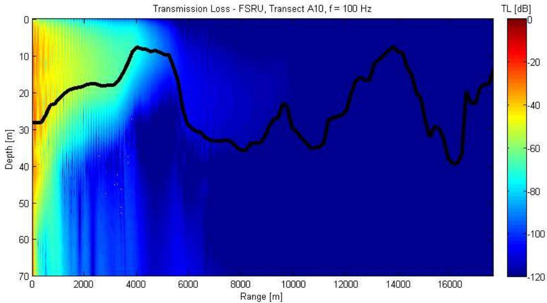
**Figure 16. Transmission loss along transect A10 at 100 Hz. Black line indicates seafloor.**
