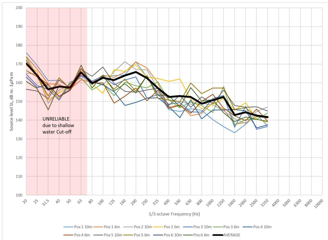
Figure 43. Measured underwater source level spectra - Golar Freeze FSRU.
