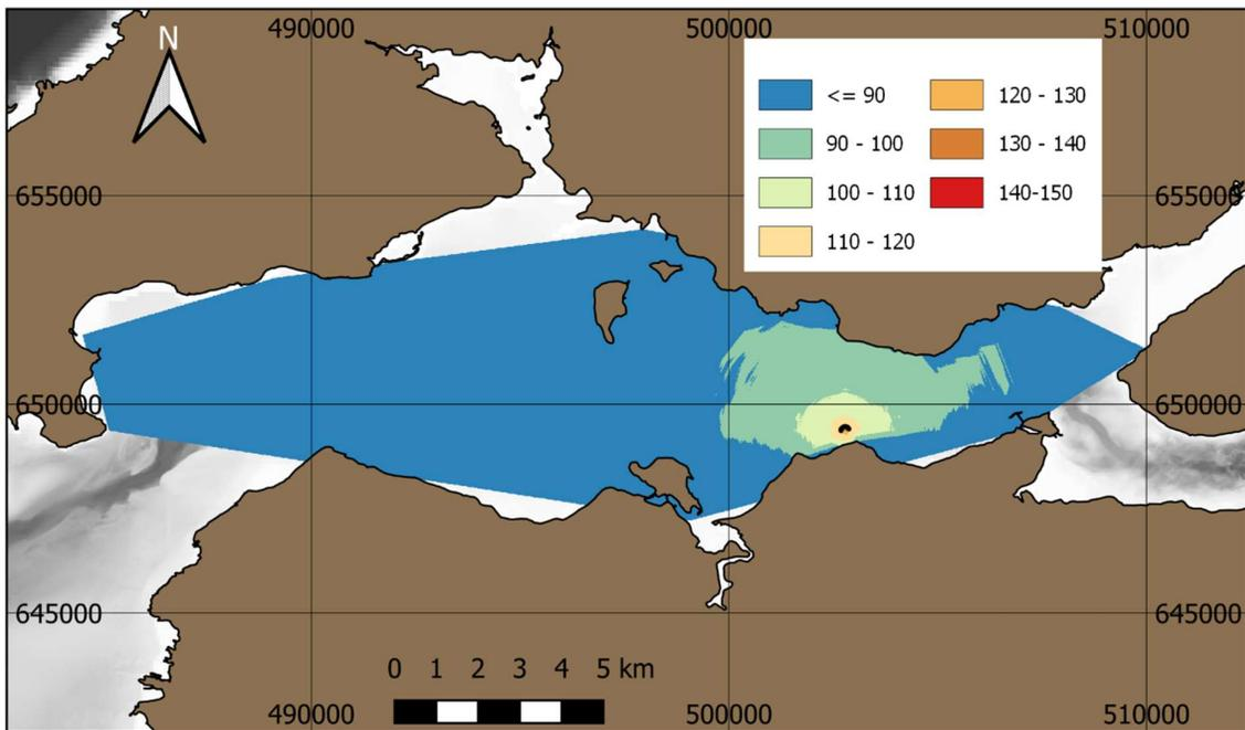
**Figure 28. Scenario C3) Construction Socket pile drilling. Contour map of  $L_{p,rms}$  (MF-weighted, "Max-over-depth"). Values in dB re 1  $\mu$ Pa. Behavioural criteria of 120 dB is indicated by dashed line.**
