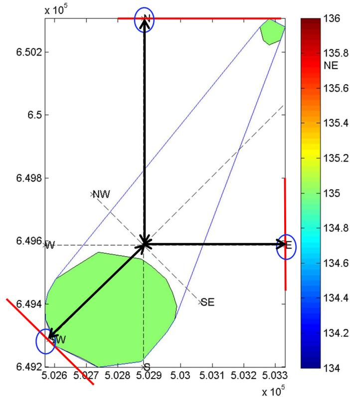
Figure 19. Example for calculation of Distance-to-Threshold for complex multiple source scenarios, shown with an example threshold of 135 dB.
