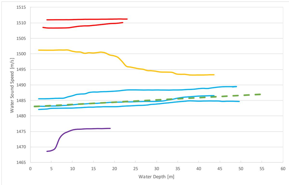
**Figure 4. Sound speed profiles in water. Dashed green line is the profile applied for the underwater acoustic modelling. See the text for other colours.**
