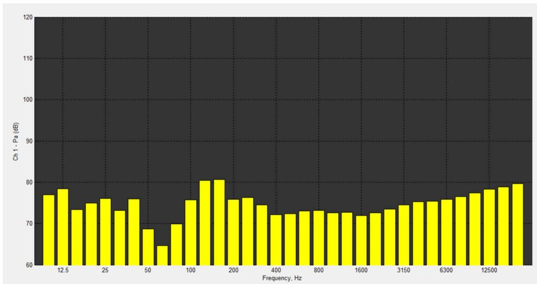
**Figure 10. Typical 1/3 octave frequency band spectrum, NIGHT – No audible ships ( $L_{p,rms}$ , unweighted dB re 1  $\mu$ Pa)**
