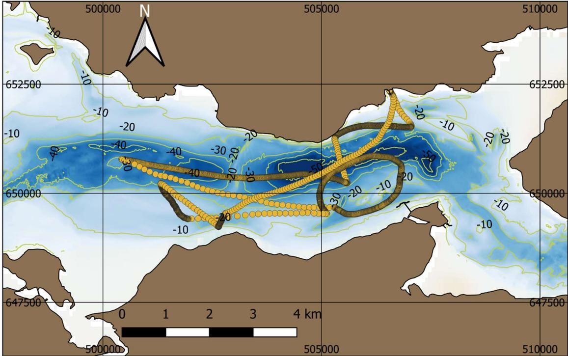
**Figure 7. GPS track of ambient noise measurements. For source of bathymetry data, see Section 2.1. Land polygons ©OpenStreetMap contributors [1].**
