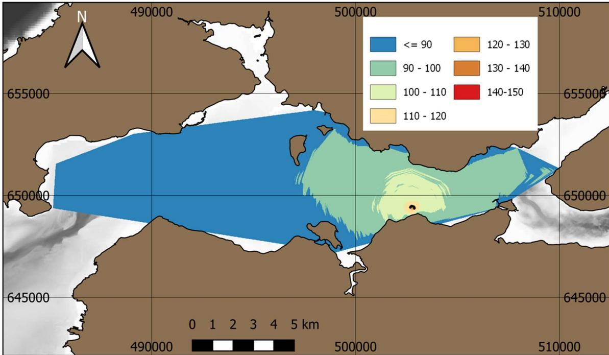
Figure 33. Scenario B) FSRU together with an offloading LNG carrier, including 1 tug in idling mode. Contour map of  $L_{p,rms}$  (MF-weighted, “Max-over-depth”). Values in dB re 1  $\mu$ Pa. Behavioural criteria of 120 dB is indicated by dashed line.
