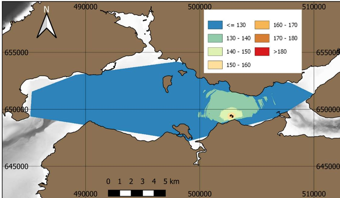
**Figure 26. Scenario C1) Construction Impact Pile driving. Contour map of  $L_{p,rms}$  (MF-weighted, “Max-over-depth”). Values in dB re  $1 \mu Pa$ . Behavioural criteria of 160 dB is indicated by dashed line.**
