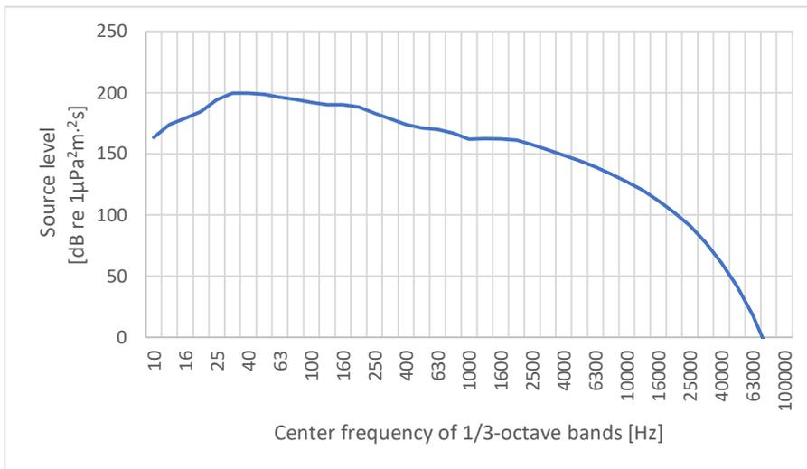
**Figure 24. Source level 1/3-octave spectrum for blasting event, stated as  $L_{S,E}$ .**
