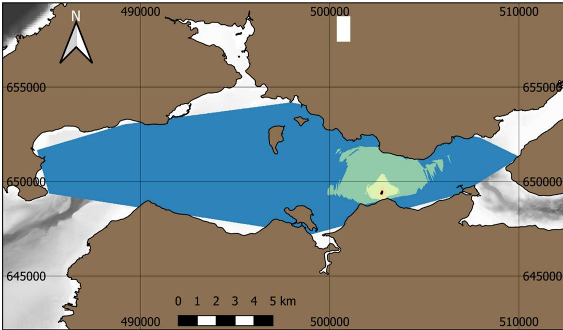
**Figure 27. Scenario C2) Construction Vibratory driving incl. supporting vessels. Contour map of  $L_{p,rms}$  (MF-weighted, "Max-over-depth"). Values in dB re 1  $\mu$ Pa. Behavioural criteria of 120 dB is indicated by dashed line.**
