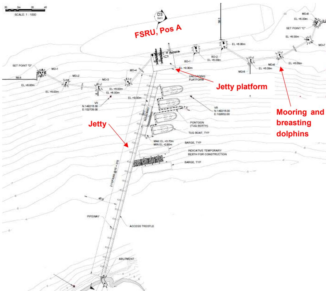
**Figure 3. LNG import jetty and Floating Storage and Regasification Unit (FSRU). Pos A, corresponding to the FSRU location, is the source location used for the acoustic modelling, see Figure 1.**
