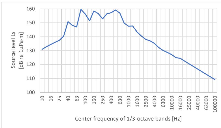
**Figure 22. Source level 1/3-octave spectrum for socket drilling,  $L_s$  dB re 1  $\mu$ Pa·m.**
