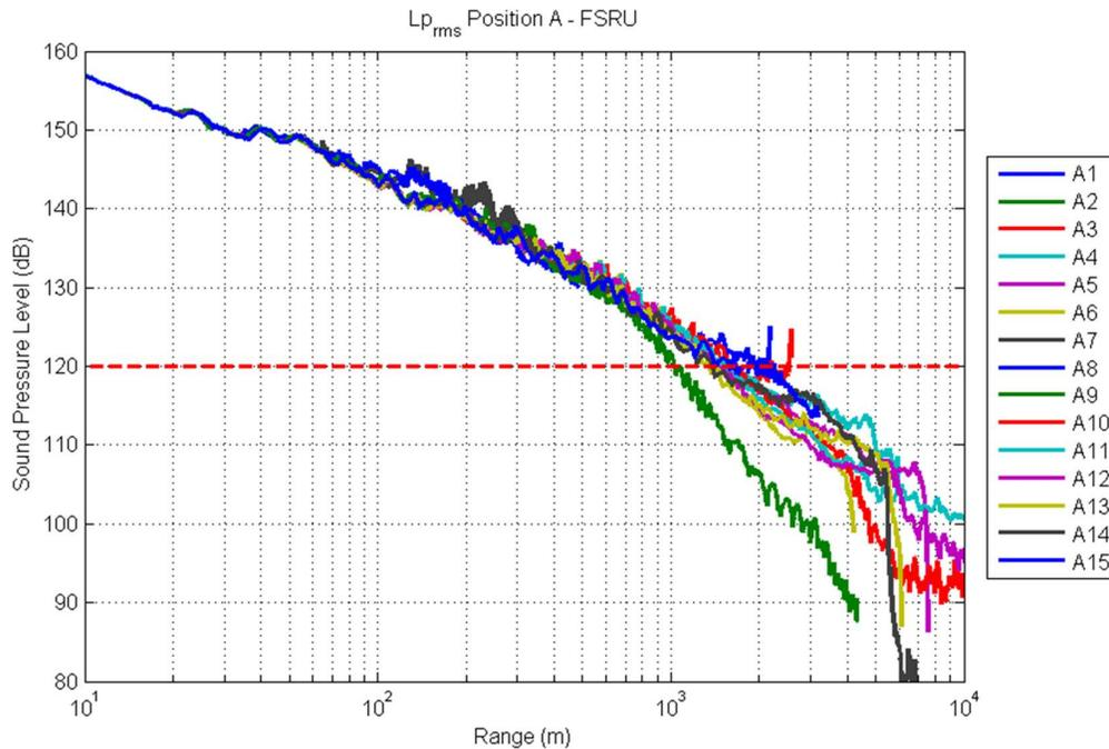
**Figure 18. Max-over-depth of flat-weighted RMS sound pressure level  $L_{p,rms}$  for FSRU.**
