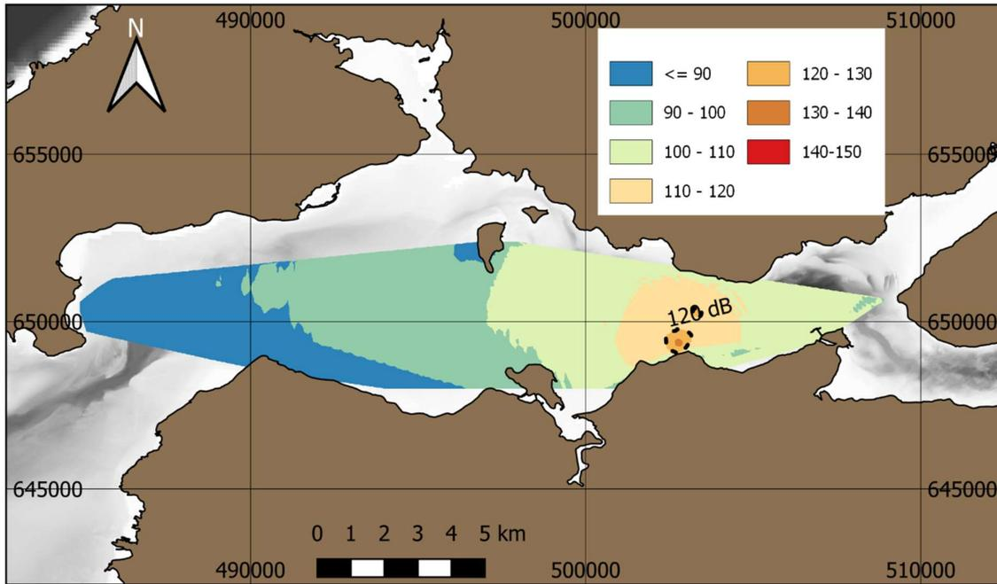
**Figure 35. Scenario E) FSRU together with berthing LNG carrier, including 4 idling /engaged tugs, a general cargo ship sailing in the middle of the Estuary, and ship moored at Moneypoint. Contour map of  $L_{p,rms}$  (MF-weighted, “Max-over-depth”). Values in dB re 1  $\mu$ Pa. Behavioural criteria of 120 dB is indicated by dashed line.**
