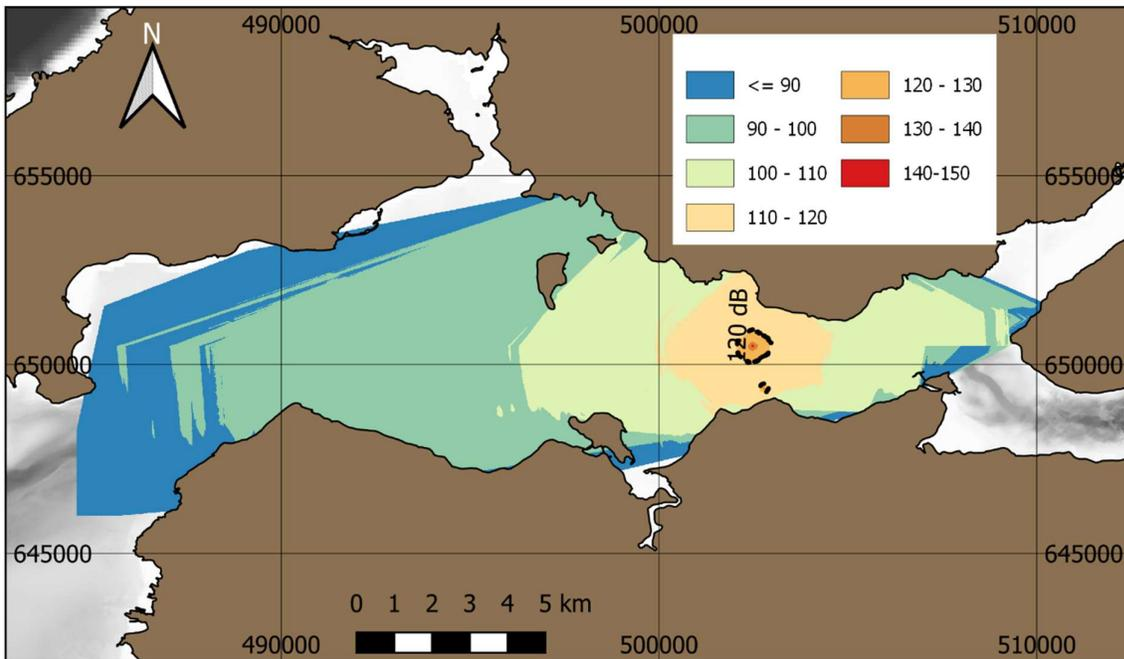
Figure 34. Scenario D) FSRU together with approaching LNG carrier, including 4 sailing tugs. Contour map of  $L_{p,rms}$  (MF-weighted, “Max-over-depth”). Values in dB re 1  $\mu$ Pa. Behavioural criteria of 120 dB is indicated by dashed line.
