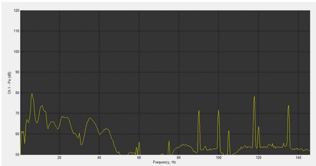
**Figure 11. Typical narrowband frequency band spectrum, NIGHT - Distant engine audible in recording - possibly generator – peaks seen in spectrum ( $L_{p,rms}$ , un-weighted dB re 1  $\mu$ Pa, Hanning window, 10 Hz HP filter)**
