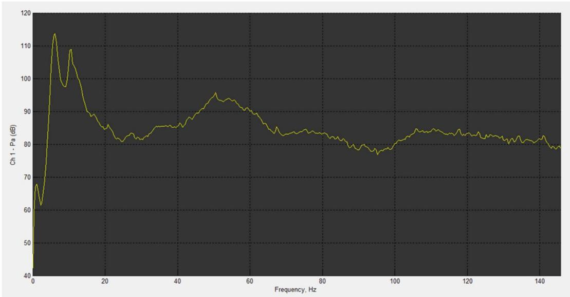
**Figure 9. Typical narrowband frequency band spectrum, DAY - Ferry 200 m away crossing from Killimer to Tarbert ( $L_{p,rms}$ , un-weighted dB re 1  $\mu$ Pa, Hanning window, 10 Hz HP filter)**
