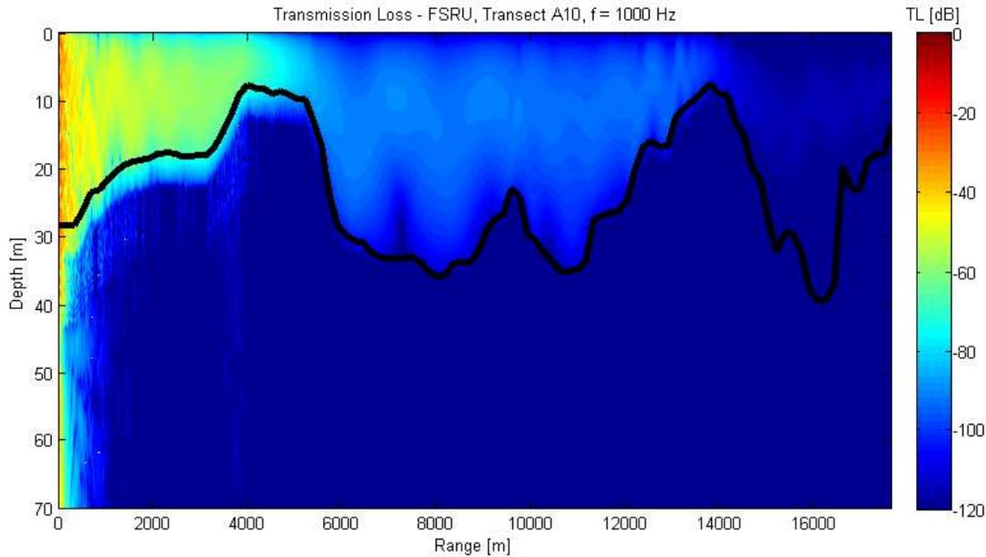
**Figure 17. Transmission loss along transect A10 at 1 kHz. Black line indicates seafloor.**
