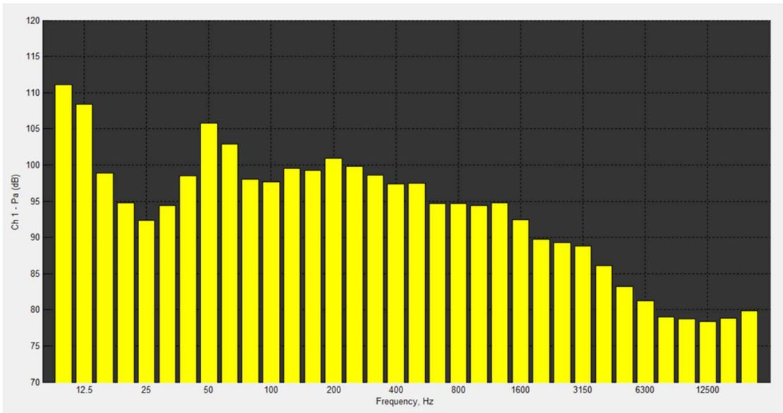
**Figure 8. Typical 1/3 octave frequency band spectrum, DAY- Ferry 200 m away crossing from Killimer to Tarbert ( $L_{p,rms}$ , unweighted dB re 1  $\mu$ Pa).**
