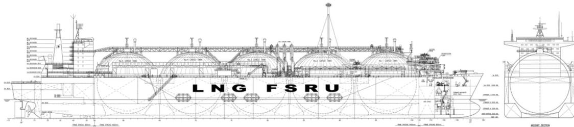
**Figure 37. Side view and section of the Golar Freeze FSRU.**
