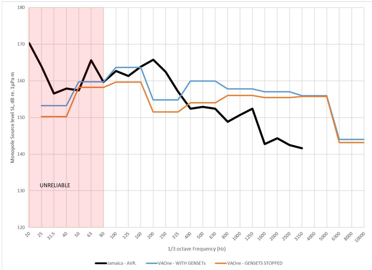
**Figure 45. Predicted underwater source level for the hull-radiated noise from FSRU Golar Igloo, compared to the measurements on the Golar Freeze FSRU measured in Jamaica.**
