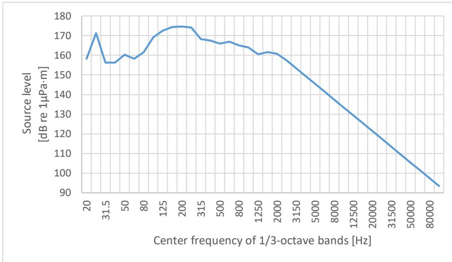
**Figure 21. Source level 1/3-octave spectrum for vibro-driving,  $L_s$  dB re 1  $\mu$ Pa·m.**
