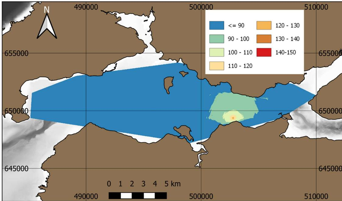
**Figure 29. Scenario C4) Blasting. Contour map of  $L_{p,rms}$  (MF-weighted, “Max-over-depth”). Values in dB re 1  $\mu$ Pa. Entire sound field is below the behavioural criteria of 160 dB.**
