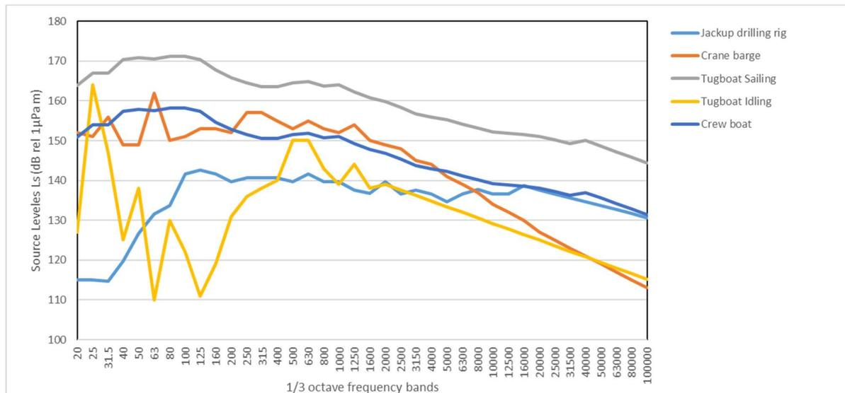
**Figure 25. Underwater source levels for support vessels used in the predictions ( $L_s$  dB re 1  $\mu\text{Pa}\cdot\text{m}$ ).**
